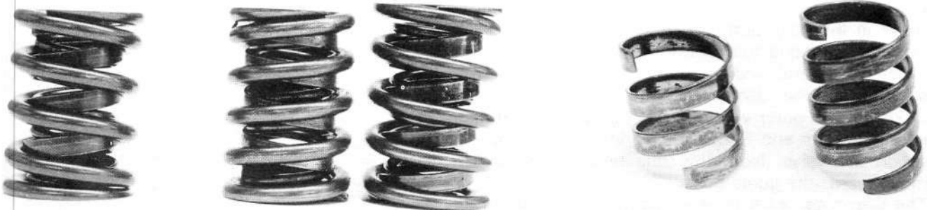
These are our current spring choices. The GK 2017 (left) works well to 0.750-inch net lift with a light exhaust valve. The GK Pro Stock spring (center) or the Norris "Battleship" winding made from Carpenter steel will work on the intake. For Nascar the GK 2001 or 2002 will do.
