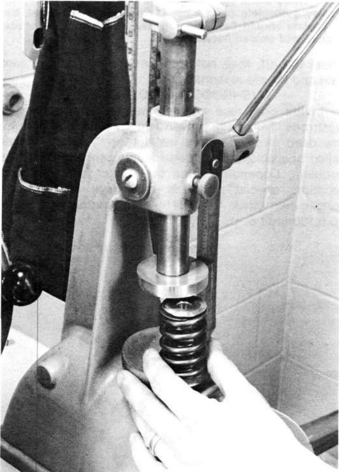
The intake springs are installed with about 180 lb on the seat to give 600 lb over the nose. They sag after initial installation and require reshimming. The exhaust springs are set at 140 lb.
