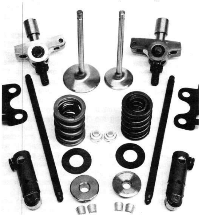
All components of a very high-rpm valvetrain must be carefully selected. A Pro Stock smallblock must turn 9,500-10,000 rpm and such speeds put exceptional demands on every single piece. Big springs, roller rockers and lifters are required.
