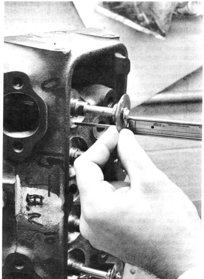
Once the seat and valve-open pressure heights are determined they must be compared with the seat-to-retainer height of the selected valves to determine the amount of seat shim required.
