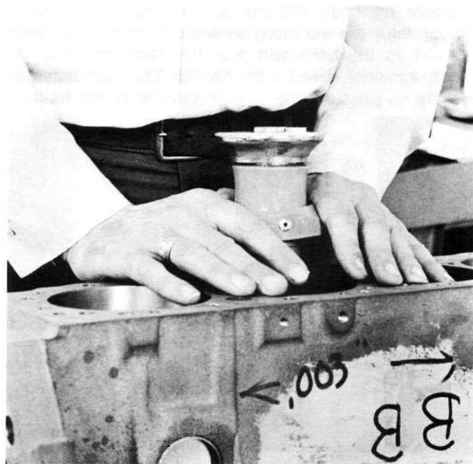
Our latest efforts have been directed toward hardness testing potential block selections. There is some variation in the production casting material and we use a portable Brinell tester to find "hard" blocks.
