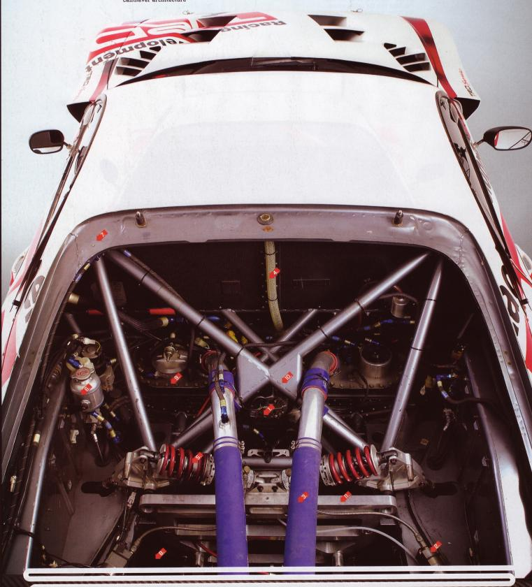
"THE CHASSIS HAS BEEN SEPARATED BY A MIX OF ROLL CAGE TUBING AND A FULL CARBON FIBRE FIREWALL.
