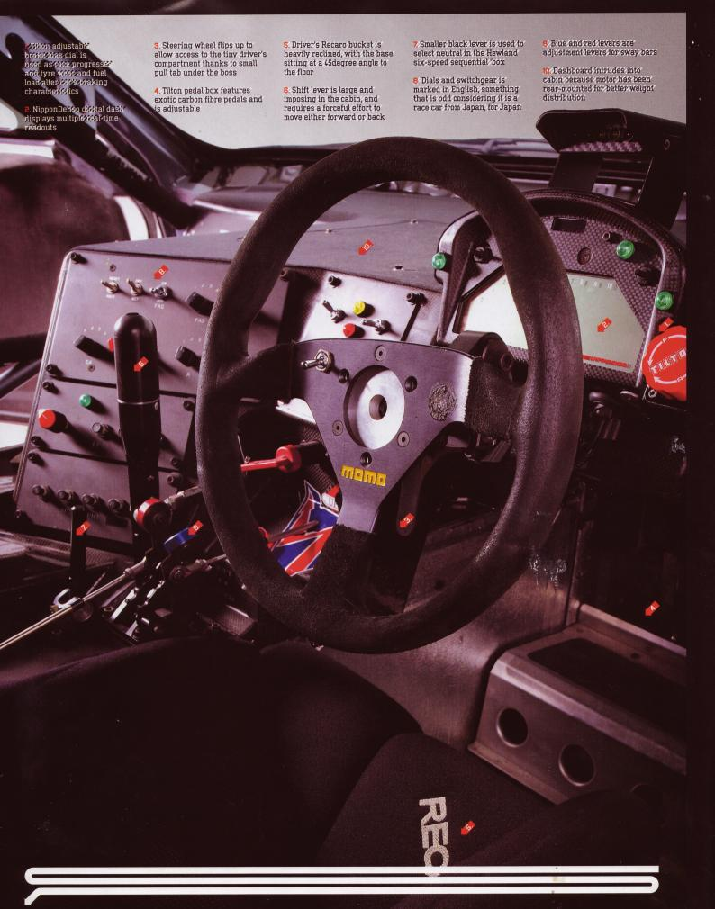
"MOUNTED TO THE FLOOR IS A MEGA-EXPENSIVE TILTON PEDAL BOX, WITH ADJUSTABLE CARBON FIBRE PEDALS.
